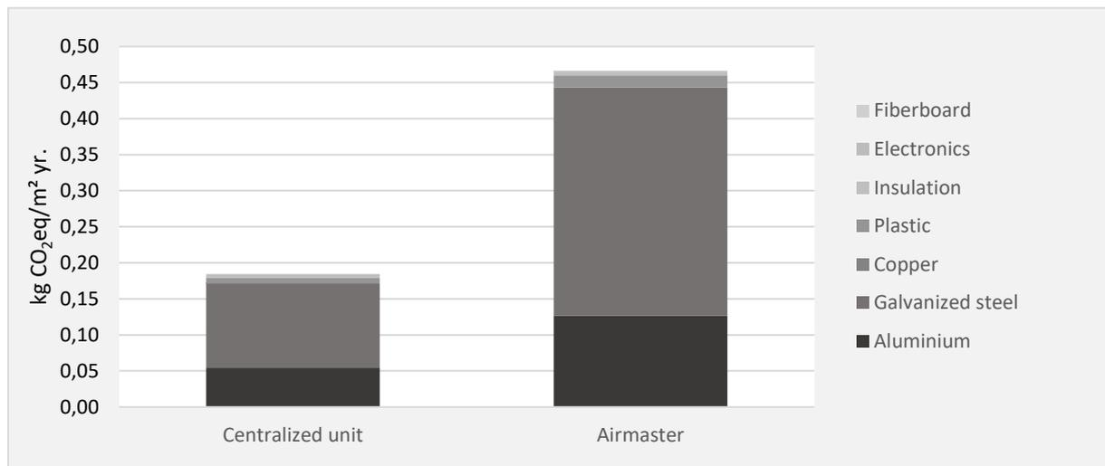
Figure 5. Total CO<sub>2</sub> emission for air handling units divided between materials.
