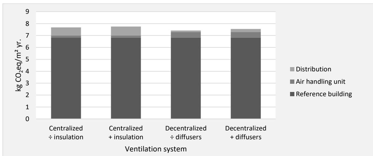
Figure 6. CO<sub>2</sub> emission for ventilation systems and reference building.
