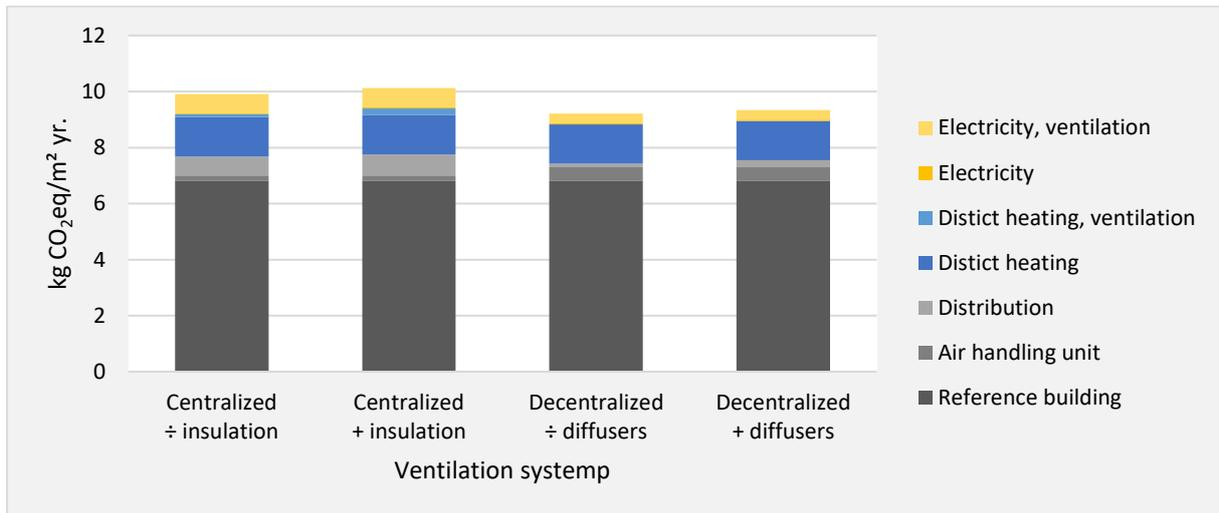
Figure 7. CO<sub>2</sub> emission for ventilation systems, reference building and operation energy.
