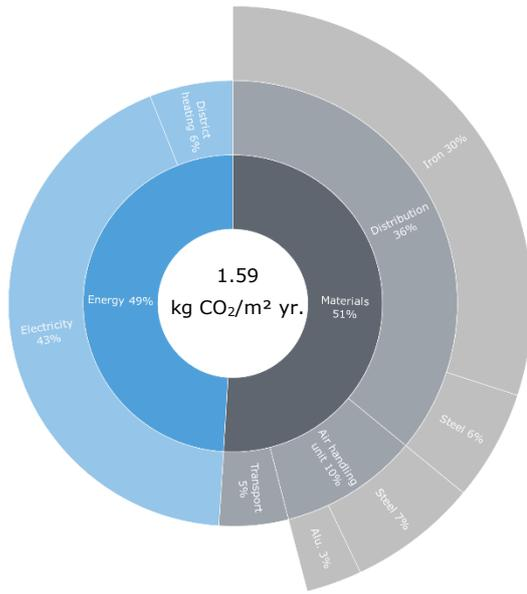
Centralized ventilation system ÷ insulation
