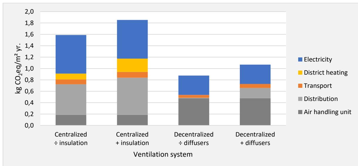
Figure 3. Total CO<sub>2</sub> emission for centralized and decentralized ventilation systems.
